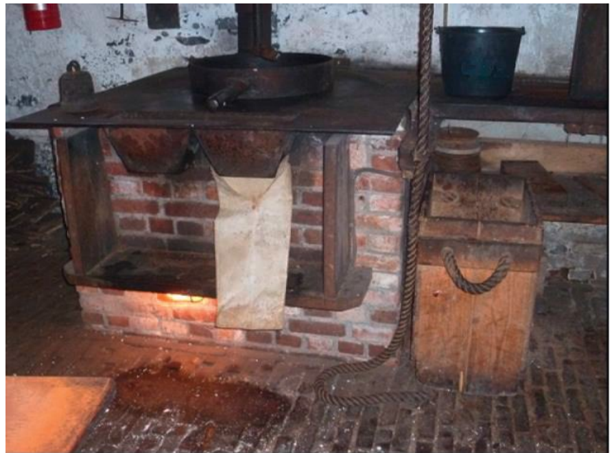
Fig. 14.2.4.2 An oil seed heater with slide ring, hoppers and a cloth bag. Oostendorper Mill – Haaksbergen
