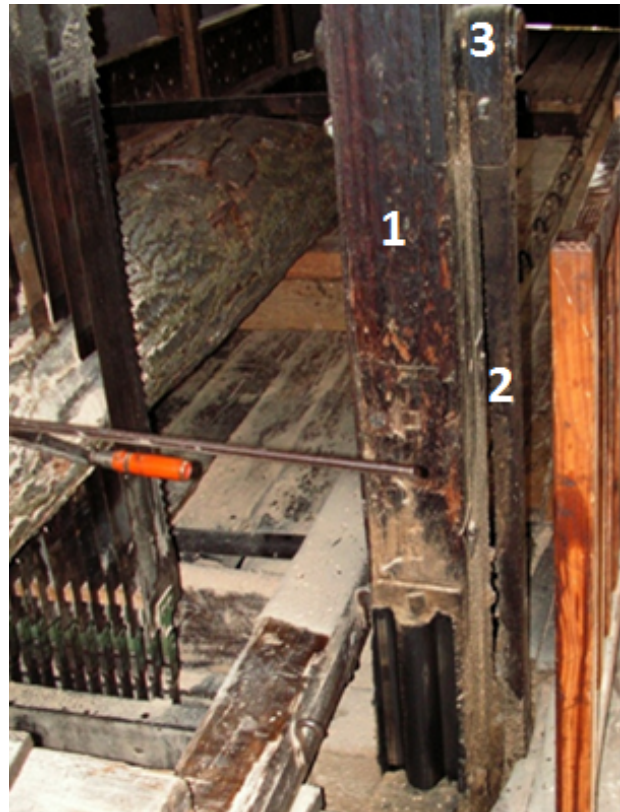
Fig. 15.2.2.4 Drive of a vertical saw frame On the right along the upright (1) is the top of the connecting rod (2) and its attachment to the frame (3)
