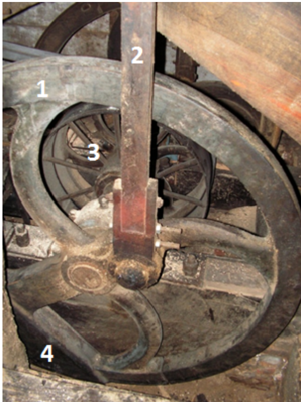
Fig. 15.2.2.3 Drive of a vertical saw frame One of the crank wheels (1) with a connecting rod (2). Behind it are the loose and fixed belt pulleys (3). Bottom left of the crank wheel is the counterweight (4).
